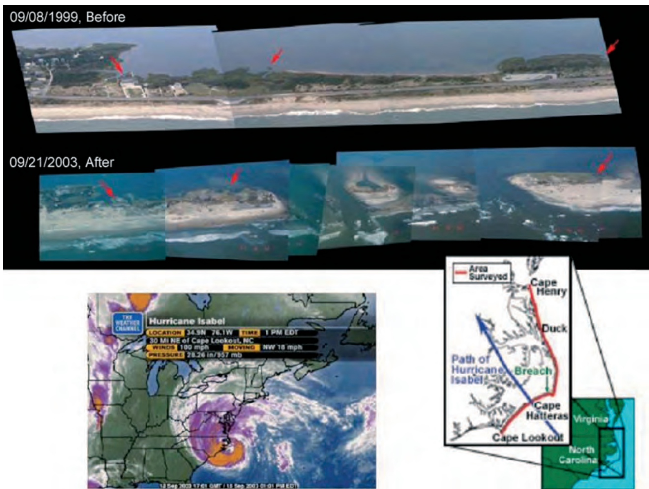
Figure 4. Hurricane Isabel struck the North Carolina coast on 18 September 2003. Upper frame: The new inlet that was cut by Isabel’s storm surge and overwash of Hatteras Island. Shown are before and after images (courtesy of USGS). Lower left frame: NOAA rainfall intensity image showing Isabel making landfall near Drum Inlet on the Outer Banks. Lower right frame: Hurricane Isabel’s northwesterly track across the Pamlico Sound after making landfall.
