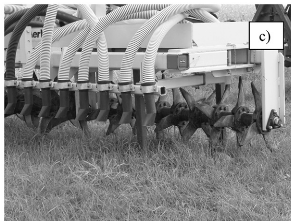
Fig. 1. Examples of novel manure application technologies currently available, including (a) a disk injector system that is capable of injecting liquid manure to a depth of 15 cm; (b) chisel injector with sweeps, which includes a disk to cut surface residue; and (c) an aerator set up to band liquid manure over the injection slots.
